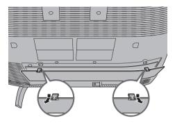
• Leave the cover off if they do not fit properly. Do not force to replace the cover. Doing so may cause damage to the connection cables and the cover.
